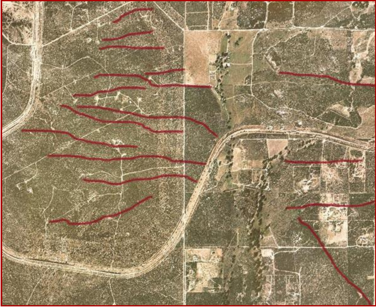
Fig. 3 Major photogeologic lineaments in the vicinity of the Campo landfill site ( Ponce, 2006 ).
