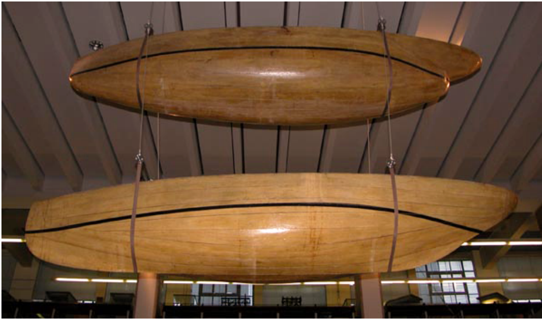
Fig. 1 The hulls of Swan (above) and Raven (below) on display at the Science Museum, London. The models were built by Froude to establish resistance and scaling laws for ship design.
